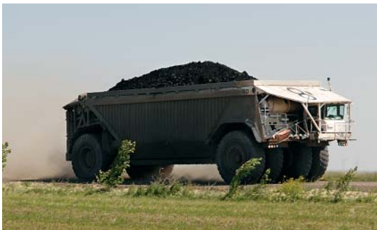
Lignite coal is loaded into 180- to 240-ton haulers and transported directly to the plant site. New 240-ton trucks will be needed beginning in 2014.
