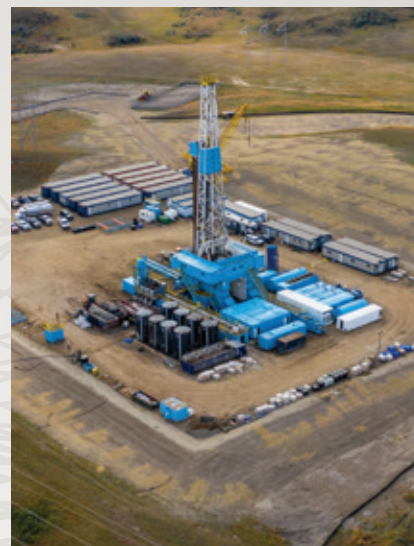
Test wells were drilled in 2020 to ensure the proposed storage zones were suitable for CO 2 storage.
